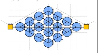
The developed prototype is of micro-drone dimensions weighing in the proximity of 160 g and employing rotors with propeller diameters of only 55 mm. This very realization of the model is suitable for reconnaissance tasks due to the small visibility footprint of the tiny aircraft and its superior noise characteristics.
